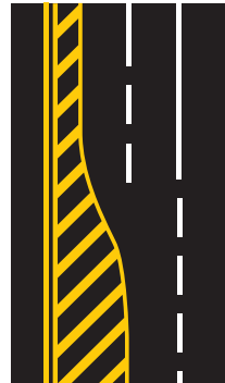
Painted island — keep to the right and do not drive on or over
