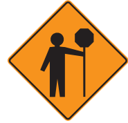
Traffic-control person ahead
